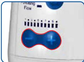
*Use + and - controls to set the desired flow rate.*
